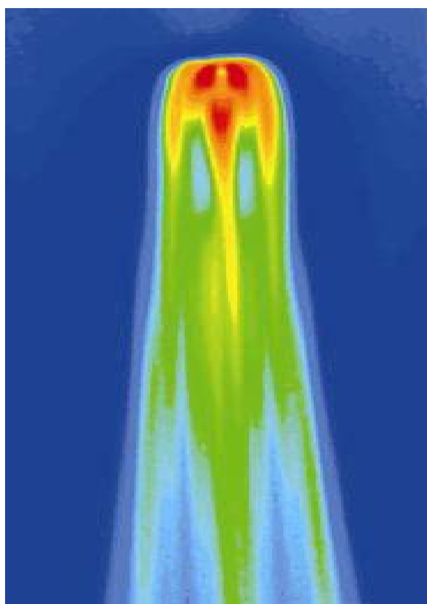
IR image: Hypersonic ( M=6 ) flow passing a square obstacle (2002)
